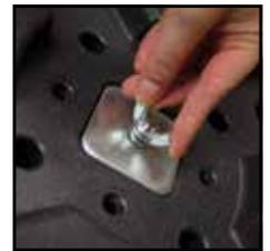
Place the assembled pole onto the revolving spigot. If required, before attaching the pole, place the required amount of stackable concrete bases onto the cross base.
